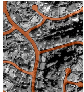
Planimetric street vector (orange, traced from aerial orthophoto) overlaid on panchromatic IKONOS satellite image (1-meter cell size) of part of La Jolla, California. Left, georeferenced but unrectified image. Right, image after RPC orthorectification, resulting in excellent match with street vector. Area has about 60 meters of relief.
