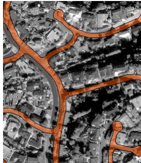
Planimetric street vector (orange, traced from aerial orthophoto) overlaid on panchromatic IKONOS satellite image (1-meter cell size) of part of La Jolla, California. Left, georeferenced but unrectified image. Right, image after RPC orthorectification, resulting in excellent match with street vector. Area has about 60 meters of relief.
