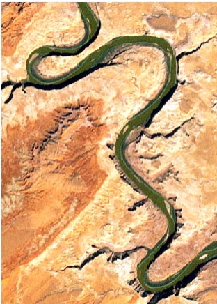
The sample GeoTIFF file is a 24-bit color composite image of the Green River in Utah, USA. This natural-color image is an extract of a pan-sharpened Landsat 7 ETM image.
