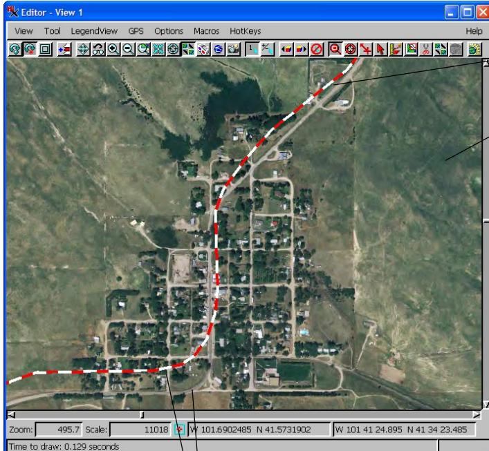
Nebraska Highway 92 fits poorly with this orthophoto image of the city of Arthur (above). The orthophoto is a WMS layer from the Nebraska Land Viewer atlas, which is provided as one of the sample atlases on MicroImages' web site. The highway line, which is a local layer, was selected for editing and vertices were dragged to fit the highway in the image (right).
